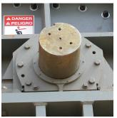
Rotor bearing housings machined by Harris from forged steel, with internal lube connection. Fittings are only needed on the
