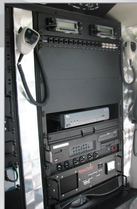
19" electronic rack with CPU, stored monitor, patch panel and Direct TV receiver.
