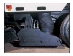
The Mechani-Pneumatic Powerhood<sup>SM</sup> option puts the A7000 in direct competition with mechanical broom sweepers for most sweeping applications. However, the A7000 is more economical to operate and provides superior removal of the PM-10 fines that are targeted as pollutants by the EPA and other agencies.
