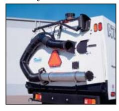
An optional, rear-mounted auxiliary hand hose is available for the A7000. It's ideal for catch basin cleanout, or for any other application where
