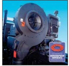
between light and heavy sweeping conditions. Connecting the fan system to the sweeping head are 14 inch diameter blast and suction tubes constructed of wire-reinforced, 3/8 inch thick molded rubber. To help ensure long fan life, the blast air goes through a selfdumping dust separator prior to reentering the 1-800-879-7933 fan housing.
