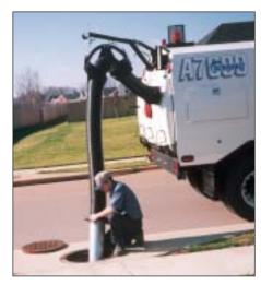
it great for a wide range of remote cleaning applications. The auxiliary hose, with its optional hydraulic controls for the hose's support boom and a four foot extension tube, makes the A7000 one of the most versatile and cost-effective pieces of cleaning equipment in the marketplace.
