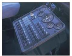
for the safety lights, optional controls and each sweeper function. The panel also includes a tachometer, an hourmeter and gauges for water temperature and oil pressure.
