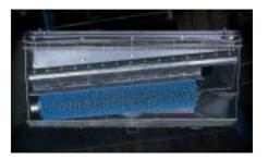
positioned ahead of the air blast to thoroughly brush the pavement surface. This broom-forward head design is ideal for loosening debris and moving it across the head. The 66 inch long, 12 inch diameter broom transfers debris toward the 14 inch suction tube, leaving the finer materials for the high pressure blast orifice.
