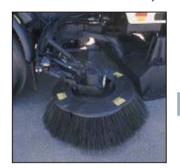
eliminate excessive wear, and prevent the possibility of gutter broom breakage due to striking an obstacle.
