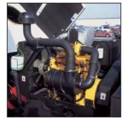
A 3-point automatic shutdown system eliminates the potential for engine damage due to low coolant level, high coolant temperature or low oil pressure. These factors help ensure a long service life for the Schwarze A7000's John Deere auxiliary engine.
