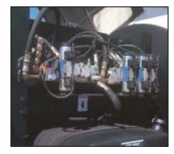
Standard operation produces a fluid flow rate of 6.5 gallons per minute. The large 25 gallon hydraulic reservoir has a 12,500 BTU cooler, which decreases oil temperature and extends the life of the hydraulic pumps, torque motors, hoses and fluid.
