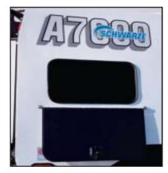
To provide fast and complete unloading, the A7000's hopper door is full height, full width, and unlatches and opens hydraulically. These features make interior hopper maintenance easier and safer for the operator. To ensure a quick, stable dumping operation, twin cylinders safely raise the hopper to a 53 degree angle. Use of 4" by 16" cylinders has reduced the standard dump cycle by 35%. The dumping operation may be controlled from either inside or outside of the cab.
