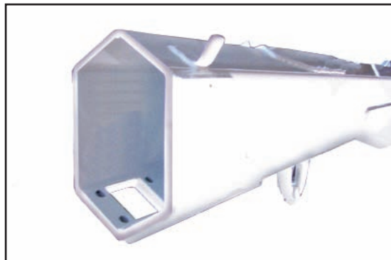
Above: Hexagonal boom construction provides a stronger cross section than square tubing. This reduces boom flex and side to side movement.
