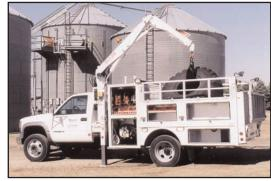
access inside the compartment. Also featured on the 1184 AG body is a left fold-down rack, and optional wheel well lights. The body of the 1184 AG features a drop-down floor to give a low center of gravity for the 400 gal. calcium chloride tank. This allows for maximum storage of the tank, maximum hauling space for the tires, and eliminates any interference with the crane.
