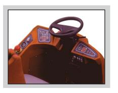
The Admiral 40's convenient operator control panel constantly monitors operations. A cushioned operator seat with a built in safety switch and a 5-position tilt steering wheel enhance operator comfort.
