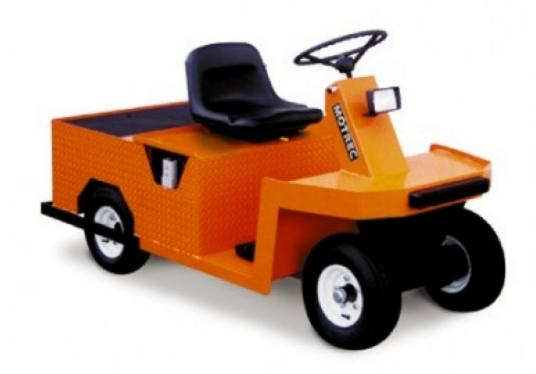
The E-290HD tractor handles the tough jobs, towing loads of up to 20,000 lb.
