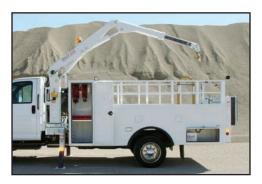
The 1302 OTR truck is mounted on a chassis cab with a 108" cab to axle and can be equipped with either a model 2200 or 3200 hydraulic knuckleboom crane. Both of these cranes are designed to handle the largest of farm tires and the smaller sized OTR tires. These cranes are both operated by a standard fully proportional radio remote control.
