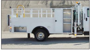
Above is a 26" vertical cabinet as shown from the passenger's side. Note the large adjustable shelves and the heavy-duty reinforced door design with stainless steel hinges. All door hardware is bolted on with stainless steel bolts and lock nuts. The optional road service strobe light is located on the top of the crane.
