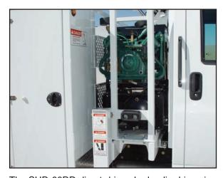
The SHD-66DD direct-driven hydraulic-drive air compressor is mounted to a 20-gallon air tank on the crane base. This compressor has a 46 CFM at 175 PSI output. The location allows for cool, clean, fresh air intake, and easy maintenance and serviceability. The SHD-66DD carries a 2-year warranty because of these features.
