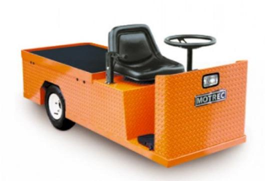
The E-272 burden carrier is engineered for tight industrial settings and jobs requiring a long deck for more cargo space.
