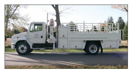
The Stellar Aggressor 138-215 MS (Mid-Size) OTR series features a rugged, heavy duty 15' steel OTR service body with over 80 cubic feet of storage. The user friendly design with the front mounted vertical compartments are standard. Each underbody compartment comes with slide top doors equipped with stainless steel automotive style slam latches.
