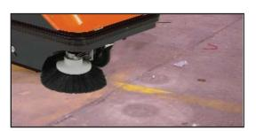
**Side brush:** The side brush throws debris into the path of the main broom. It is excellent along curbs, skids and racks.
