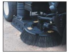
Schwarze's industry-leading *Gutter Broom Extension Override*<sup>®</sup> (*GEO*<sup>®</sup>) system enables the brooms to scrub directly in front of the head.
