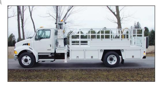
The Stellar Aggressor 138-15 MS (Mid-Size) OTR series, features a rugged, heavy duty 15' steel OTR service body with over 60 cubic feet of storage. The standard driver side rail folds down, for ease and safety of loading and unloading of tires, as well as sign boards for identification.
