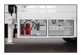
The SHD-66DD direct-driven hydraulic-drive air compressor is mounted on the crane base. model SHD-66DD direct drive hydraulic air compressor is a 4-cylinder, 2-stage compressor with a 100 cubic inch displacement and an output capacity of 46 CFM @ 175 PSI The crane boom is stored in travel position in a unique crane saddle, which will ease wear and tear on the turntable bearing. The SHD-66DD carries a 2-year warranty because of these features.
