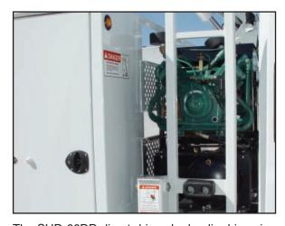
The SHD-66DD direct-driven hydraulic-drive air compressor is mounted to a 20-gallon air tank on the crane base. This compressor has a 46 CFM at 175 PSI output. The location allows for cool, clean, fresh air intake, and easy maintenance and serviceability. The SHD-66DD carries a 2-year warranty because of these features.
