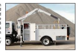
The 1302 LCF OTR truck is mounted on a chassis cab with a 108" cab to axle and can be equipped with either a model 2200 or 3200 hydraulic knuckleboom crane. Both of these cranes are designed to handle the largest of farm tires and the smaller sized OTR tires. These cranes are both operated by a standard fully proportional radio remote control.
