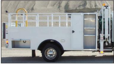
Above is a 26" vertical cabinet as shown from the passenger's side. Note the large adjustable shelves and the heavy-duty reinforced door design with stainless steel hinges. All door hardware is bolted on with stainless steel bolts and lock nuts. The optional road service strobe light is located on the top of the crane.
