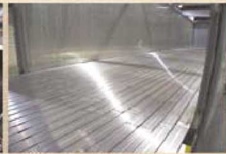
The slat latching device engages, connecting dock to trailer.
