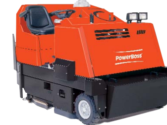
Monitor 82 & Monitor 90 Double Scrubbers Up to 77,500 sq. ft. per hr (7,200 sq. m.) * 42" - 60" Sweeping Path (106 - 152cm) 42" - 48" Scrubbing Path (106 - 152cm) 68 - 100 Gal Solution Tank (257 - 379 L) 65 - 100 Gal Recovery Tank (246 - 379 L) Disc or Cylindrical Brush Available Gasoline, Diesel or LP Powered *spec based on 90
