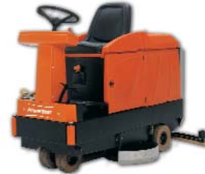
Admiral 36 Rider Scrubber 57,000 sq.ft. per hr (5,300 sq. m.) 35" Scrubbing Path (88cm) 37 Gal Solution/Recovery Tanks (140L) Battery Powered
