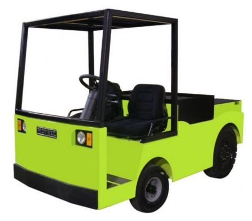
T-8000 is engineered for safe in-plant towing of a 50,000 lbs load. Its width is similar to a lift truck, to maneuver in the same space.
