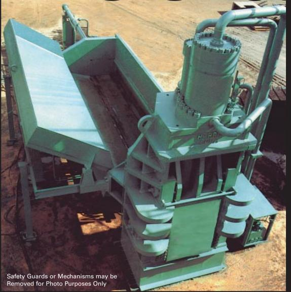
Developed with an emphasis on economy, the Harris line of ABS shears has proven to be fast and economical, meeting the needs of scrap processors around the world. ABS employs a unique concept in design; a pre-compression charging box in which one half of the box opens to accept scrap, and the other half remains rigid with the "Tuck-and-Fold" flipper. All this plus the dependable, heavy-duty construction found in more expensive shears makes the ABS shear a wise choice for any yard.
