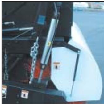
To assure contour sweeping, the cylinder lowers with no resistance. This allows the main broom to follow road contours seamlessly. The broom is driven by a hydraulic motor via an efficient chain drive system.
