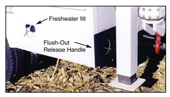
The conveniently mounted fresh water rinse tank is shown on the left, and the Stellar exclusive Flush-Out release handle on the right.
