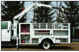
optional wheel well lights. The body of the 1184-13 AG features a drop-down floor to give a low center of gravity for the 400 gal. fluid tank. This allows for maximum storage of the tank, maximum hauling space for the tires, and eliminates any interference with the crane.
