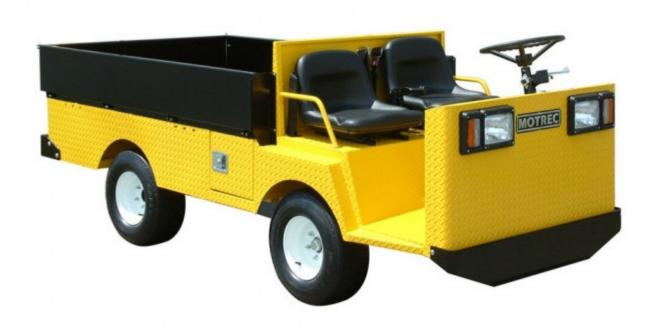
The E-480TT electric vehicle, with 18 mph speed and 3000-lb. capacity, provides an efficient replacement for gas vehicles to move around your plant. It allows you to keep pace with new environmental laws while enjoying significantly lower operating costs – like all our electric burden carriers, it requires very little maintenance.
