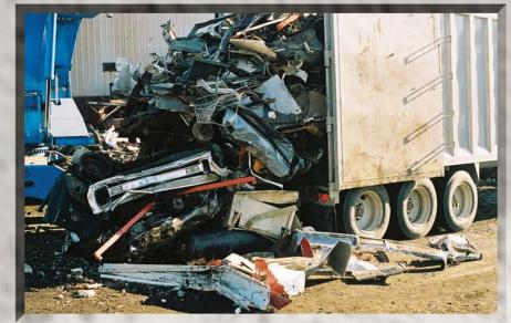
WALKING FLOOR technology is a hydraulically driven, moving floor conveyor. Floor slats extend the length of the trailer or bin floor. While in motion, the floor slats remain horizontal, reciprocating alternately and then in unison to convey the material.
