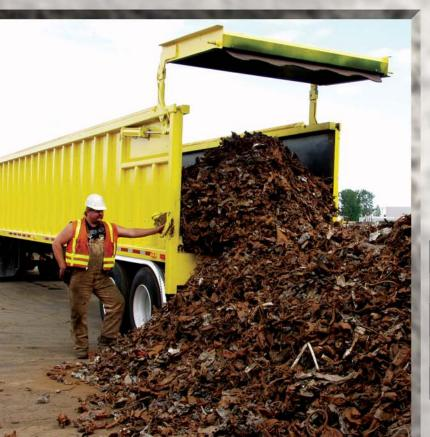
When installed in a trailer, the V-Floor unloader provides safe, efficient and versatile horizontal unloading. The system is designed for handling hot asphalt, aggregate, crushed cars and other extremely abrasive materials. Like all *WALKING FLOOR* systems, the V-Floor unloader is low maintenance and easy to operate.
