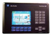
•Touch screen color display with function keys and programmable logic controller. Program has 15 material selections and programmable settings.
