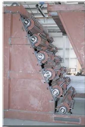
**Discharge Auger:** Conveys lumpy, sluggish material from the bin at a controlled rate.
