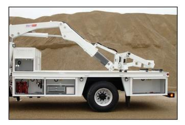
The heavy duty OTR body shown below is designed to meet the medium OTR needs. Features include underbody tool compartments with slide top doors equipped with stainless steel automotive style slam latches. Other features include D-ring tie downs, recessed skirt-mounted halogen floodlights, DuPont Imron 5000 paint, and complete body undercoating. A heavy duty frame mounted push bumper is mounted at the rear of the body.
