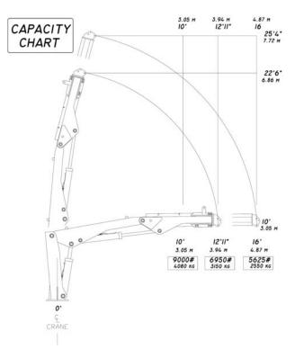
The chart above shows the lifting capacities and reach for the 9000 crane **without** the TM3107. TM3107 has a lifting capacity of 3400 lbs.
