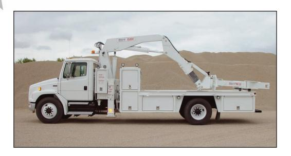
Power, Precision, Durability. That's what you get with the Stellar 15000 OTR series, designed from the ground up to work in the OTR tire service industry. A durable 320° turntable rotation system driven by a worm gear / pinion system ensures rock solid rotation performance. This crane features a lifting capacity of 15,000 lbs. at 10' and 9,000 lbs. at 16'6" of total reach, without the tire manipulator.
