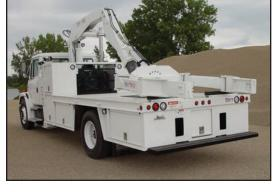
modifying the A-frame geometry and using dual cylinders we are able to allow A-frame stability at differing outrigger widths.
