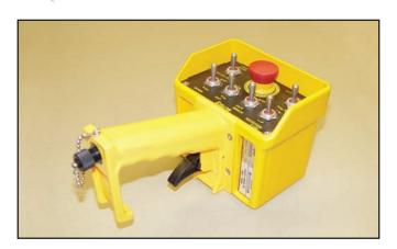
The Stellar 9000 OTR series is the only crane in its class to offer a variable speed handheld radio remote control as a standard feature. The radio remote control system allows operators to maintain a safe operating distance between themselves and the load. A push button on-off switch in the pistol grip handle ensures that the crane is activated only by the operator.
