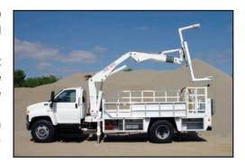
All of the underbody tool compartments come standard with the exclusive Stellar slide top doors for unobstructive storage access. Stainless steel automotive style slam latches and hardware are standard on all tool compartments.
