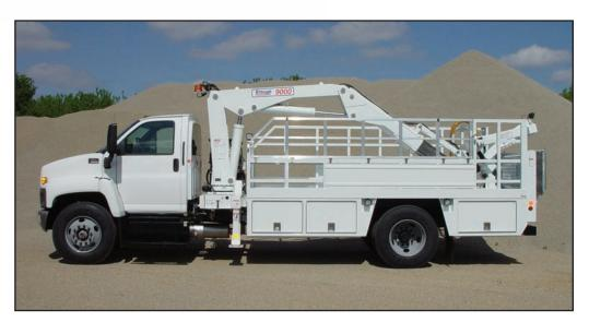
The Stellar Aggressor 9000-RS OTR series, features a rugged, heavy-duty 15' steel OTR service body with over 60 cubic feet of storage. The standard driver-side rail folds down, for ease and safety of loading and unloading of tires, as well as sign boards for identification.
