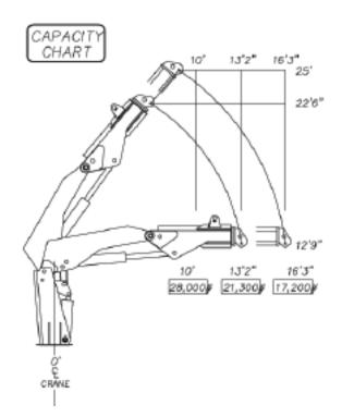
The chart below shows the lifting capacities and reach for the 28000 crane **without** the TM16160. TM16160 has a lifting capacity of 16,000 lbs.
