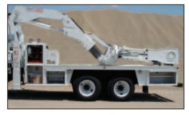
The 28000 OTR series truck has a rugged 20' heavy duty OTR body with 85 cubic feet of storage space. Each underbody compartment comes standard with slide top doors equipped with stainless steel automotive style slam latches. The storage compartment shown below is the main working compartment on the 28000/TM16160. It offers hose reels, a FLR, and tool storage at bed level and close to the working area.
