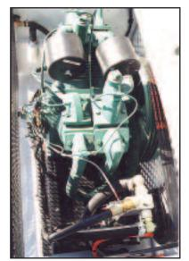
Stellar's model SHD-245 air compressor is designed to meet the heavy duty OTR tire service industry. The industrial 4 - cylinder, 2 - stage compressor is powered by a hydraulic motor and outputs 110 CFM @ 175 PSI.
