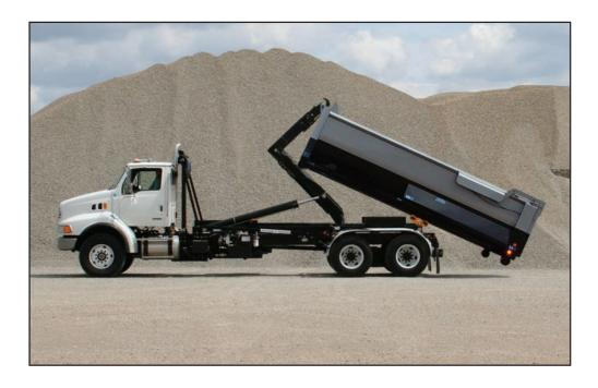
The Stellar Slider65 hooklift is a body handling system mounted on a truck chassis that is capable of loading, unloading and dumping various bodies with lengths ranging from 16' to 22' (4877mm to 6706mm) with the use of a hexagonal sliding jib. Now with an adjustable hook height, the Slider65 will handle 54" (1372mm) or 61.75" (1568mm) hook height bodies and will accommodate capacities up to 65,000 pounds. The maximum dump angle is 50° on a 41-inch (1,041mm) high truck frame.
