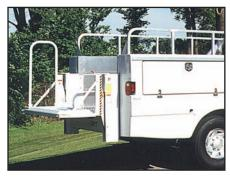
constructed of stainless steel. The use of aluminum in the frame and the use of stainless steel hardware makes this body virtually corrosion proof.
