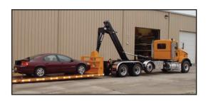
The 16,000 pound Stellar Shuttle features the new breakaway dump/tilt tabs.
