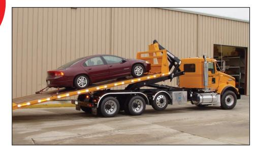
The 40,000-pound capacity Stellar Shuttle hooklift loaders are one of the most popular sizes for construction use. The shorter 108-14-40 is popular when used with a 15-foot dump body for general purpose hauling. The 138-18-40 is ideal for use with a 2,500-gallon water tank or vacuum pumper. The longer 174-20-40 and 190-22-40 models are solid values for hauling larger debris boxes or hauling heavy construction equipment, such as paving machines.
