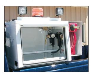
Both the SGD and SHD models come standard with a protective steel framework that houses the compressor and a driver side locking tool compartment. The entire unit is primed and painted white.
