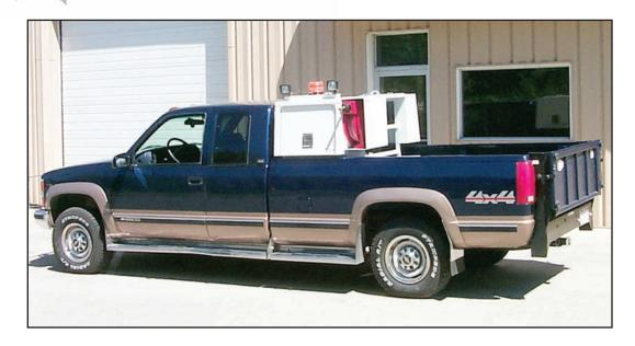
The Stellar Back-Pac Service Module is an ideal unit for metro, road and light fleet tire service applications. The Back-Pac is a self-contained steel module that can turn a full size pick-up into a service truck in a short period of time. The Back-Pac is manufactured in two models, the gas powered SGD and the hydraulic powered SHD. Both models use the same module and compartment footprint.
