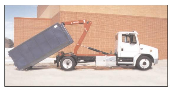
Economical, versatile and efficient, are just a few of the features offered by the Stellar Xchange Hooklift. Designed for chassis with a cab to axle of 108" to 120", the Xchange is by far the simplest hooklift in the marketplace today.
