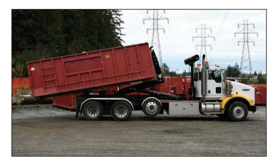
The Stellar Slider34 hooklift is a body handling system mounted on a truck chassis that is capable of loading, unloading and dumping various bodies with lengths ranging from 14' to 20' (4267mm to 6096mm) with the use of a hexagonal sliding jib. Now with an adjustable hook height, the Slider34 will handle 54" (1372mm) or 61.75" (1568mm) hook height bodies and will accommodate capacities up to 34,000 pounds (15,422kg). The maximum dump angle is 50° on a 41-inch (1,041mm) high truck frame.
