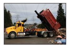
The Stellar Slider series hooklift is known for its versatile design and ease of operation. All models of the Stellar Slider feature permanently lubricated and greaseable bushings used throughout, the Stellar patented dump/load interlock system, and an efficient low flow/high pressure hydraulic system.
