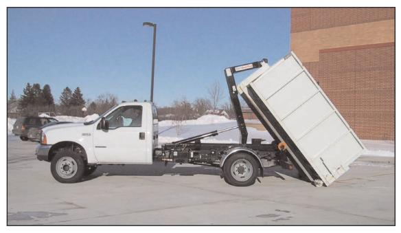
Economical, versatile and efficient, are just a few of the features offered by the Stellar Xchange Hooklift. Available in 9,000 and 13,000 pound capacities and fitting chassis with a cab to axle of 84" to 130", the Xchange is by far the simplest hooklift in the marketplace today.
