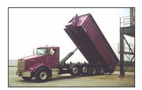
Every Stellar hooklift loader places emphasis on ease of operation. Dual controls, located inside the cab of the truck, provide a comfortable environment for the operator. Stellars unique Aframe tilting section allows full visibility of the lifting hook during container engagement. These standard features allow for greater safety and quicker cycle times during loading and unloading.
