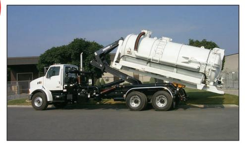
When heavy hauling is required, look to the 65,000-pound Stellar Shuttle. These models are designed to handle the extremely heavy loads of both on and off-road hauling. The Stellar 65,000-pound loaders feature dual 7-inch bore lift / dump cylinders to keep the overall height as low as possible. Dual rear rollers with integral rear body tie-downs are standard.
