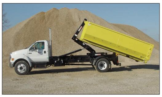
The Stellar Slider hooklift loader is a container handling system mounted on a truck chassis that is capable of loading, unloading and dumping various containers with lengths ranging from 12' to 18.5' with the use of a sliding hexagonal jib. The hex jib reduces flex and provides greater structural integrity. The Stellar Slider can accommodate capacities up to 20,000 pounds. The maximum dump angle is 55° with a 54" hook height on a 41-inch high truck frame and below grade capabilities to 46".
