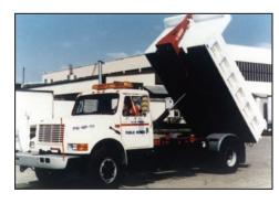
As with all Stellar hooklift loaders, simplicity of design and operation are a top priority. All our loaders feature permanently lubricated greaseless bushings, our patented dump/load interlock system, and an efficient low flow/high pressure hydraulic system. Gravity type safety latches are used to prevent accidental detachment of the body, while rugged rear body tie-downs insure body
