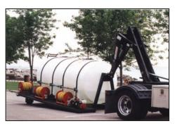
stability when in transit. Only Stellar hooklifts provide a full length dump frame with front saddles to support the body during the dump mode. These are just a few of the standard features incorporated into every Stellar hooklift loader.
