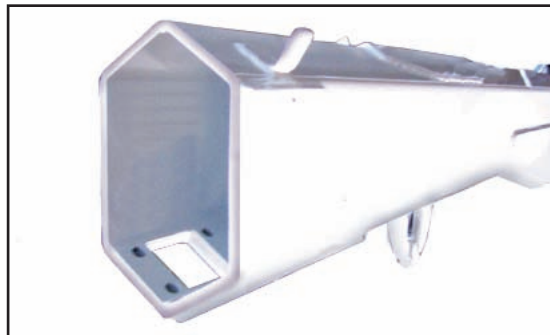
Above: Hexagonal boom construction provides a stronger cross section than square tubing. This reduces boom flex and side to side movement.
