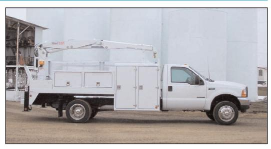
The Class 1 & 2 LP Gas Service Trucks from Stellar Industries, Inc. are extremely versatile service trucks. They make transporting, loading and unloading gas cylinders a simple, single-person operation without the need of a trailer or additional setting equipment.
