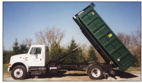
Stellar's line-up of 20,000-pound capacity hooklift loaders offer the greatest selection of any hooklift manufacturer. With five different lengths available, the 20,000-pound Stellar Shuttles cover from 102" to 190" cab-to-axle lengths for single rear axle truck chassis.
