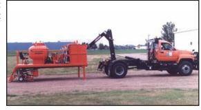
loading and dumping without the use of springs, sliding rods, rotating cams, or electric switches. Stellar Industries is the only manufacturer in the world to offer this unique design as an integral part of their hooklift loader.
