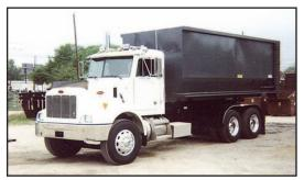
As with all Stellar Shuttles, simplicity and operation are a top priority. All Stellar loaders feature permanently lubricated greaseless bushings, a patented dump/load interlock system, and an efficient low-flow/high-pressure hydraulic system. Gravity type safety latches are used to prevent accidental detachment of the body while rugged rear body tie-downs insure stability.
