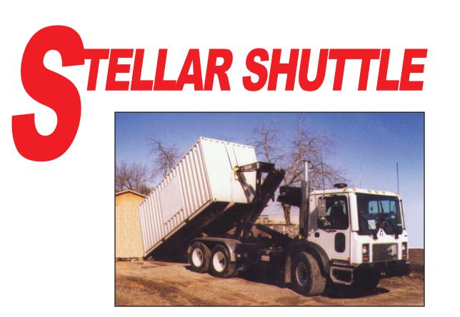
With a 34,000 pound capacity and a 54" hook height, this model of hooklift was designed to facilitate hooklift owners who need a greater load capacity. Even with increased capacity this Stellar Shuttle does not require changing the hook height on existing containers.
