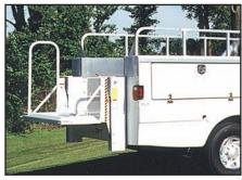
The Stellar Model EDL-54 powered liftgate can lift loads up to 1,300-pounds and features a hydraulic cylinder lift. For those applications where a liftgate is not desired, an attractive steel pickup style tailgate is available with a rear step bumper and body-mounted hand grab rails.
