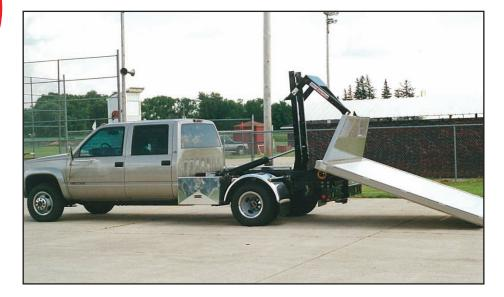
The Light Duty Hooklift is designed to provide the construction contractor, landscaper or municipal user with expanded uses not available with a standard pick-up box. Dump boxes, flatbed bodies, and small water or fertilizer tanks can easily be pulled up onto a Shuttle equipped truck.
