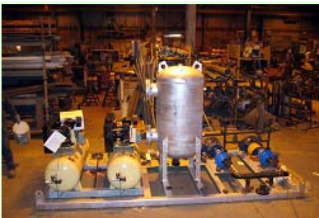
Saturator Vessel Skid under manufacturing
