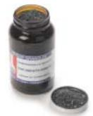
Carbon boiling chips are chemically inert to concentrated sulfuric acid, strong alkalies, and other chemicals. Carbon chips can be used for atmospheric or vacuum operations. Silicon carbide (carborundum) chips are random-sized pieces up to 2 mm long.
