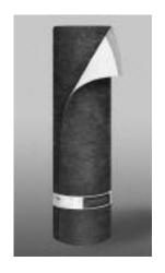
**Product Use:** FLINTGLAS CAP SHEET COOLSTAR is a roll roofing product designed for use as a cap sheet over inorganic and organic built-up roofing systems. FLINTGLAS Mineral Surfaced Roof Systems are suitable for both new construction and reroofing applications over a variety of substrates. It is surfaced with ceramic granules and an acrylic-based CoolStar coating to provide a durable, heat reflective weathering surface when used as a cap sheet.
