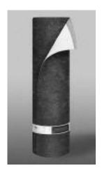
Product Use: FLINTLASTIC FR-P COOLSTAR is designed for use as a roofing membrane cap sheet in SBS modified bitumen roof system assemblies over various types of substrates for both new construction and reroofing installations. It is suitable for most low slope roofing applications and may be used for roof system flashings including wall treatments, base flashings and field flashings.
