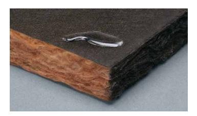
ToughGard 2 is more moisture resistant than standard duct liners thanks to its unique enhanced surface. Moisture that enters the duct system beads up and stays beaded, allowing airflow to evaporate the moisture before it can be absorbed into the liner. A drier duct environment lessens the chances that mold will be an issue, and improves the quality of the air that is transmitted through the ducts.
