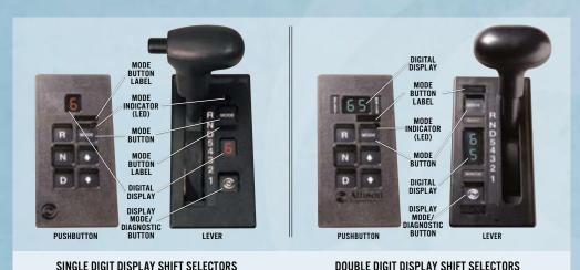
Vehicle manufacturers may choose different types of shift selectors for their vehicles. The shift selector in your Allison-equipped vehicle will be similar to one of the pushbutton or lever styles as shown above.
